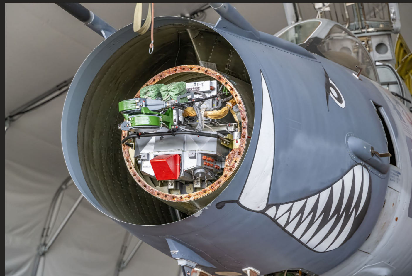
Klyon-54 Laser targeting system/-designator / image by: Robert Kysela
