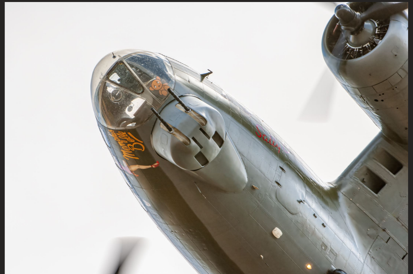
Remotely controlled chin turret / image by: Robert Kysela
